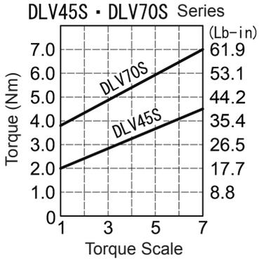
Range of use of speed level and output torque (for reference)
