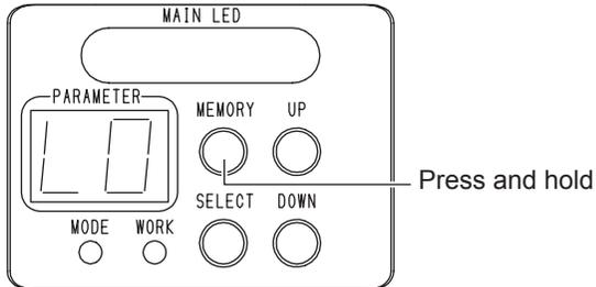
The parameter LED displays "LO" and the keys are locked.
