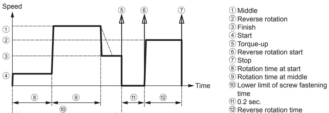
\* Stop at the lower limit of screw fastening time
