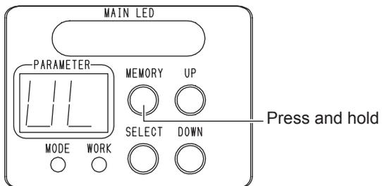
The parameter LED displays "UL" and the keys are unlocked.
