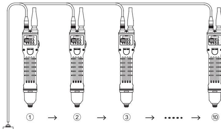
Electric screwdrivers start in order of connection and when the set screw count is reached, the next connected electric screwdriver becomes operable.
